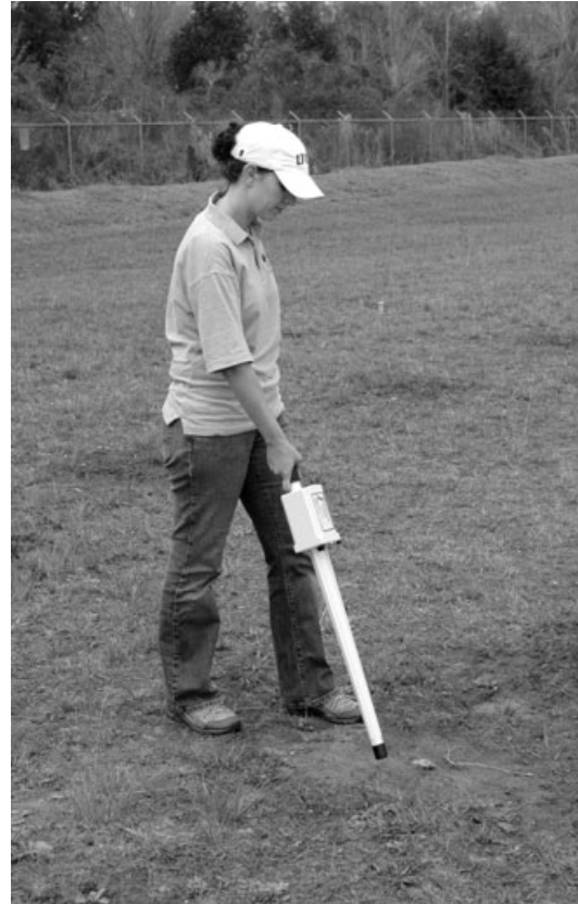
FIG. 1—Schonstedt GA-72Cd® magnetic locator being used for data collection in the field.
